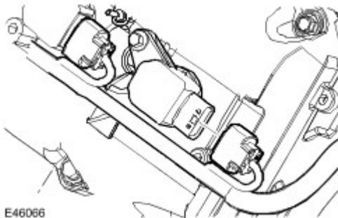
5. Remove the ignition coil-on-plug.
