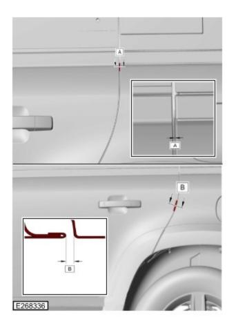
Check the alignment of the rear door(s) in the areas shown in the illustration.
