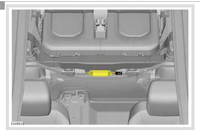
Remove the 2 Mild Hybrid Electric Vehicle (MHEV) battery cooling duct clips.
