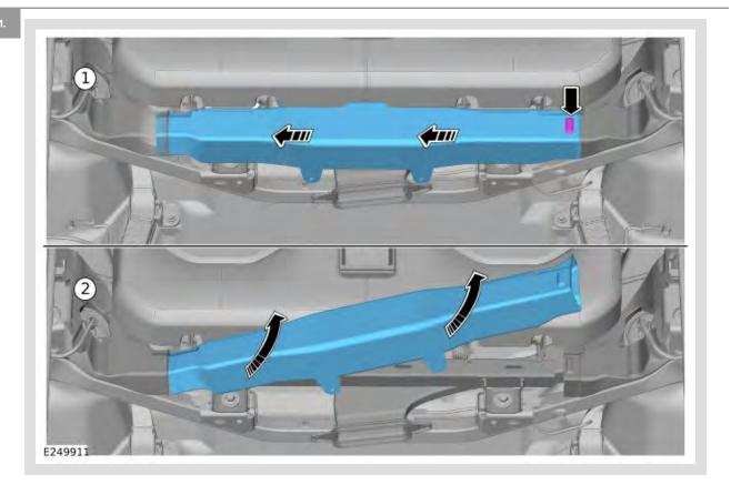
Release and remove the third row seat footwell air duct as illustrated.
