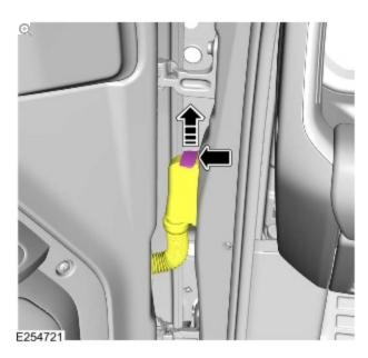
Disconnect the front door wiring harness from the body wiring harness.
