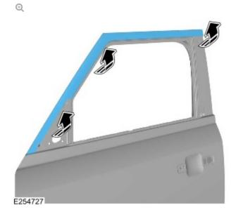
Remove the front door frame upper finisher.
