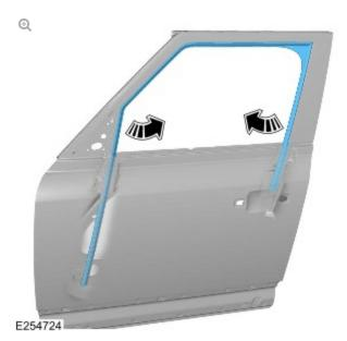
Remove the front door window runner seal.
