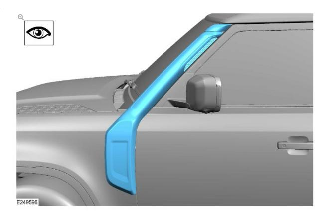
Make sure the raised air intake is correctly installed.
