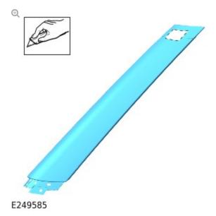
Use suitable tooling to cut the A-pillar trim as illustrated.
