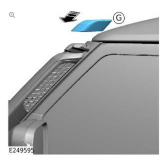
Install the cap (G) to the raised air intake.
