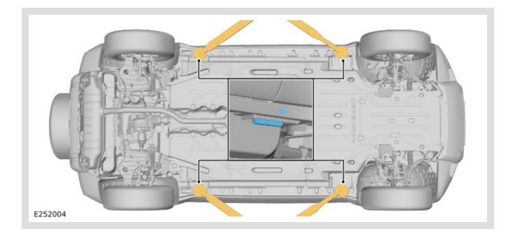
1. Position the vehicle with the center of the lift pillars aligned approximately with the front of the front row seat base cushions.
