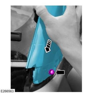
Apply downward pressure onto the windshield molding and fully tighten the retaining bolt.
