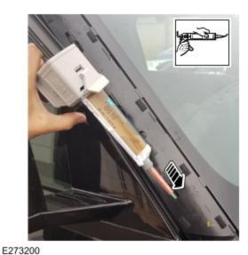
Using the recommended adhesive and applicator, apply the adhesive in the bottom of the slotted holes.
