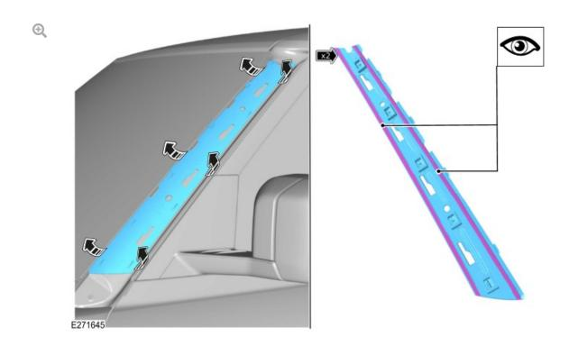
Check that the 2 strips of double sided tape are fully adhered to the body.
