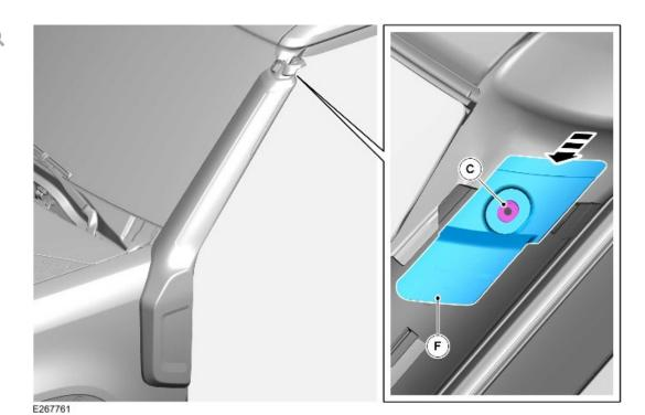
Install the bracket (F) into the slot in the raised air intake.
