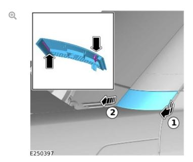
Release the 2 clips to remove the left windshield molding bolt cover.
