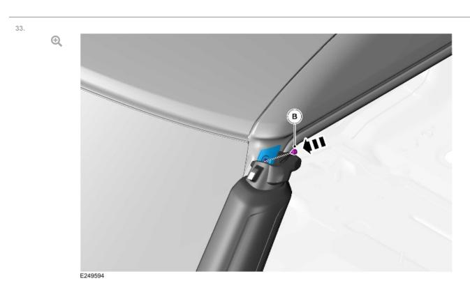
Install the bolt (B) through the bracket and into the fixing.
