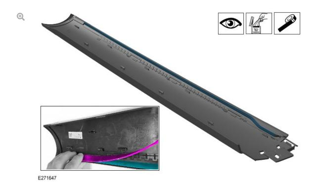
Inspect the rubber seal on the windshield molding for damage. If the seal is damaged a new windshield molding is required before continuing with this step, this must be claimed as a separate warranty claim.
