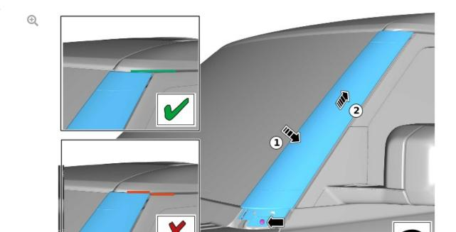
Install the windshield molding in the directions shown in the illustration.
