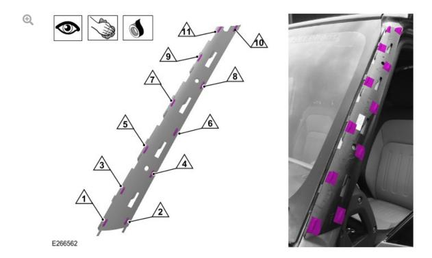
Locate the 11 windshield molding retaining ribs, as shown highlighted in the illustration.
