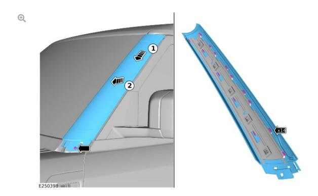
Remove the retaining bolt and then remove the left windshield molding.
