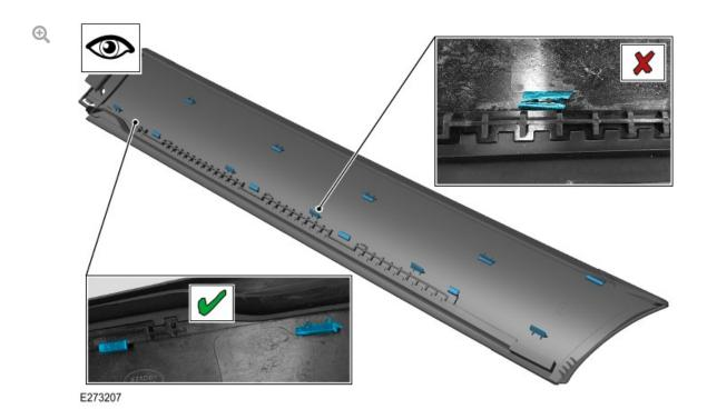
Inspect the windshield molding for damaged clipping features.
