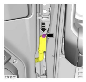
Connect the front door wiring harness from the body wiring harness.
