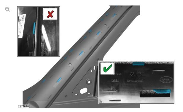
Visually inspect the windshield molding carrier for damage to the clipping features shown in the illustration.
