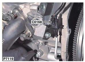
Description:Sensor-Crankshaft position (CKP) - V8Location:Rear LH side of engine
