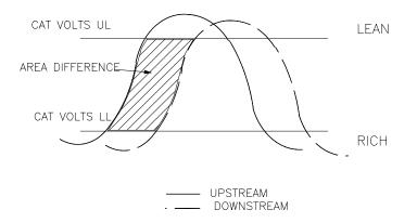
The value of CAT SUM OF DIFFS is then corrected for Air Mass Flow Rate (AMFR) by multiplying it by the following expression: AMFR /(CAT MAXIMUM AMFR - AMFR) where CAT MAXIMUM AMFR is a constant set to the largest value that AMFR can reach for that engine. The corrected value is called CAT NORM AREA DIFF.
