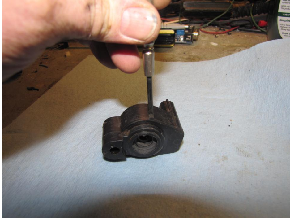
Figure 6: Opening the housing
