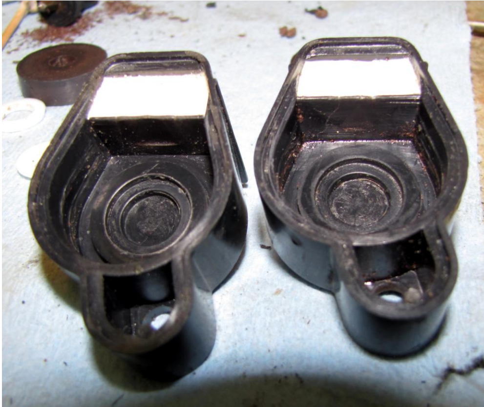
Figure 11: Two VSS housings showing wear from magnet rubbing.
