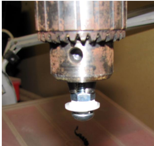
Figure 14: Tool installed in drill press
