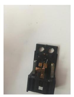
6. Lightly grease and reassemble being careful to put the springs over the white pylons and into the holes in the other half.
