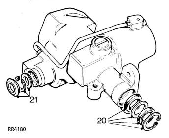
20. Remove circlip and seal from sector shaft housing bore.
