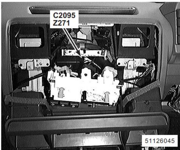
159. behind centre of fascia Z271 Engine Immobilisation Control Unit (Spider) C2095 (9-B)
