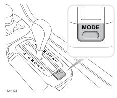
In High range press the mode switch to select 'Sport' mode (the 'S' information light on the instrument panel will illuminate).
