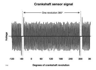
The ECM outputs an engine speed signal to the automatic gearbox, the SLABS ECU, the instrument pack and the ACE ECU. The signal to the automatic gearbox TCM and the SLABS ECU are supplied via the CAN link, while the signals to the ACE ECU and the instrument pack are carried via a frequency dependent digital signal.
