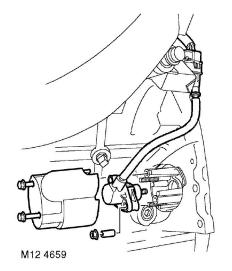
three wires attached to it; one signal wire, one ground wire connected to the ECM and one ground wire connected to vehicle ground. This last wire acts as a shield to earth any stray electromagnetic radiation produced from the crankshaft signal.
