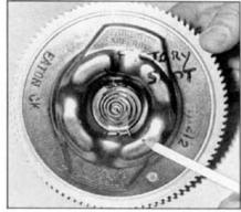
With some of these clutches, you'll be able to rotate the end of the coil all the way into the second slot using slight pressure. In others, there is no slot in the opposite tang, so rotate the spring to let the end rest against the tang. In either case, you'll get maximum cooling at lower temperatures than the factory setting.
