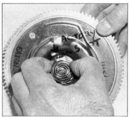
To adjust the thermostatic coil, lift the end out of the factory slot and rotate it towards the second slot. You will be rotating the valve, which turns only in the one direction when you're making this adjustment. You'll fell a lot of resistance if you try and rotate the coil in the wrong direction. You'll also notice that the valve itself will not be rotating.
