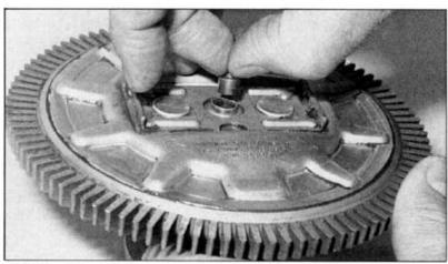
With the plate out of the way you can remove the brass plunger from the clutch.
