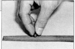
The brass pin is relatively soft, so stroke it gently along a file. Check your measurement every couple of strokes to avoid shortening too much. Don't use a grinder to shorten the pin and don't grip it with a pair of pliers or you'll burr the surface. The plunger has to slide easily in its housing. Smooth the pin with emery when you've filed it down to the correct length.
