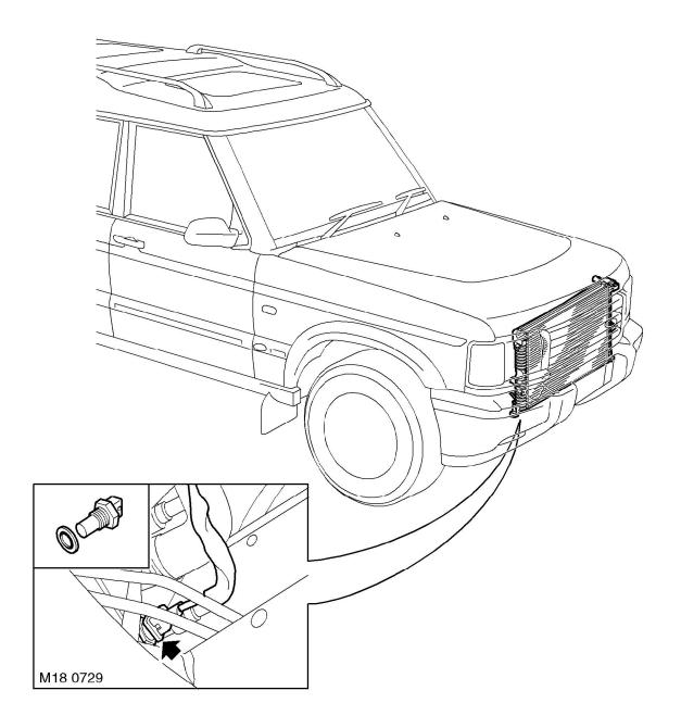
The thermostat monitoring sensor is located in the radiator, adjacent the bottom hose. The ECM compares the temperature measured by the thermostat monitoring sensor to the temperature measured by the ECT sensor. If the difference between the two readings is too great, the ECM determines the thermostat is stuck. In this case, the ECM registers a fault code in its memory.
