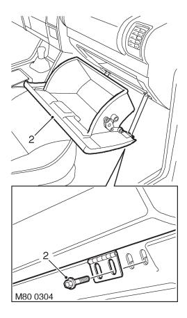
**2.** Remove 4 screws securing glove box, release catch and remove glove box.
