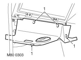
1. Remove 4 studs securing toe board and remove toe board.
