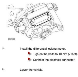
5. Using T4, calibrate a new differential locking motor.
