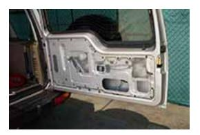
With the subwoofer removed, you are ready to move the entire inner lining of the cargo door. You need not remove the storage basket fitted to the lining. The liner is secured to the cargo door by several grommets. The grommets simply pull out. I used a large screwdriver covered with masking tape. This is not the proper tool, but will suffice if you are careful. You can see that I made a cruciform cut into the transparent film to permit access to the co-axial cable.
