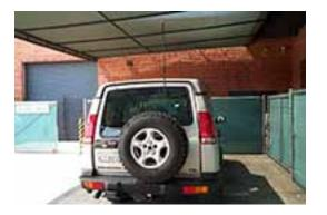
Here is a view of the competed antenna mount, with a four-foot Firestik II antenna (part no. FS4-B) fitted. This is the antenna that Han will use on the trail and on road trips.
