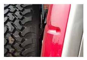
Here is a side view of the mounted antenna beside the spare wheel. There is plenty of clearance on both sides of the antenna. The antenna, when located properly, will touch neither the spare tire nor the rear wiper arm.
