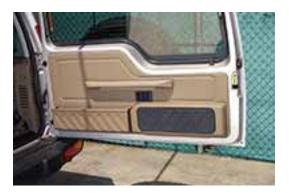
To access the co-axial cable for proper routing, you will have to disassemble your cargo door panels. If you are contemplating fitting larger than stock tires, you may want to invert your spare wheel carrier at
