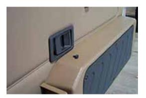
Remove the plastic cover beneath the cargo door's latch. The cover is secured by a single screw. The cargo door's handle is secured by two hex bolts that are easily unscrewed.
