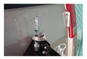
Here is a close-up view of the inside wall of the spare wheel carrier and antenna mount. Note that there is plenty of room for the co-axial cable connector. If you purchase the correct length fasteners, you should not have any problems.
