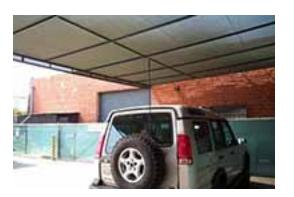
Han's Discovery II gets a lot of mileage in Downtown Los Angeles. For city use, we fitted a two-foot Firestik II antenna (part no. FS2-B). With the Quick Disconnects fitted to the antennae and the stud mount, it is a simple matter to change antennae. The shorter antenna gives clearance for parking structures and garages, but still provides adequate transmission and reception.
