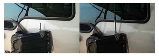
To the stud mount, we fitted a Firestik Quick Disconnect (internal locking model, part no. K-1A). This quick disconnect permits easy attachment and removal of your CB antenna. Just push the antenna onto the mount and turn the antenna to lock, what Firestik aptly describes as a "push-n-twist" system. The quick disconnect is very handy for situations when you may want to remove your antenna to avoid theft or to make clearance for entering parking structures.
