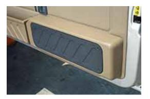
Start disassembling the cargo door panels by removing the subwoofer's screen. The screen is affixed by six screws.
