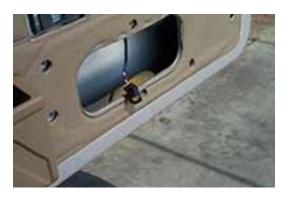
When removing the subwoofer, be careful not to yank on the subwoofer's power plug. Undo the plug and remove the subwoofer completely.
