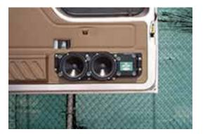
The subwoofer is secured to the cargo door by eight bolts. Unscrew all of these bolts and the subwoofer can be removed.
