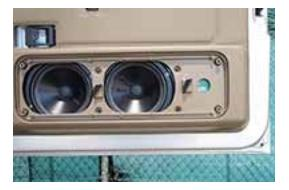
Removing the screen will expose the four screws securing the subwoofer's plastic cover. Unscrew these four screws and remove the plastic cover.
