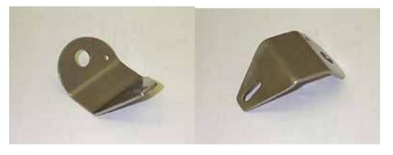
After deburring and polishing the trimmed edges, the transformed mount looks like this. To the sides and above the single remaining elongated hole, I drilled two holes through which I would place two additional mounting bolts.
