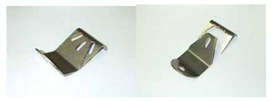
Using a cutting wheel on a Dremel tool, I removed the excess material from the mount.
