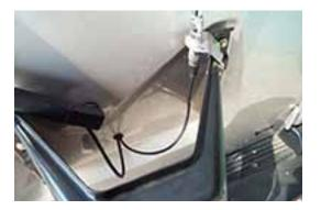
With the antenna properly mounted, it's time to route the co-axial cable. Gratefully, the Discovery II is fitted with a large rubber grommet beneath the spare wheel carrier to permit routing of the rear washer hose. We routed the co-axial cable through this grommet and did not have to drill a hole through the cargo door. The grommet is large and flexible enough to encircle the both wires without damaging the grommet.
