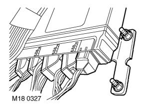
The engine control module (ECM) is located on the RH side A post below the face panel inside the vehicle. It has a cast aluminium case and is mounted on a bracket. The ECM has 5 independent connectors totalling 134 pins.
