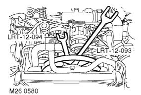
Remove viscous fan using tool LRT-12-093 and tool LRT-12-094.
