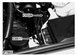
Description: *Pump-Cruise control - LHD* Location: *Rear RH side of engine compartment*
