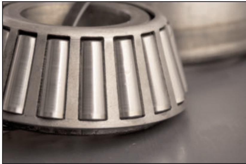
Pinion tapered roller bearing in like-new condition.
