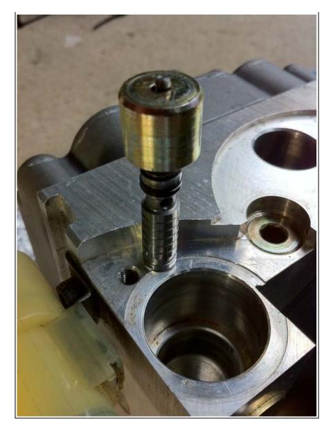
11. Install NEW circlip. (Falconworks instructions call for securing TWO circlips on each plunger)
