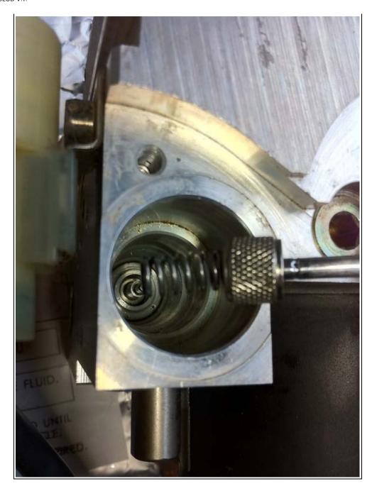
6. Use needle nose pliers (preferably with 45 degree bend) and pull upward on the plunger to remove.
