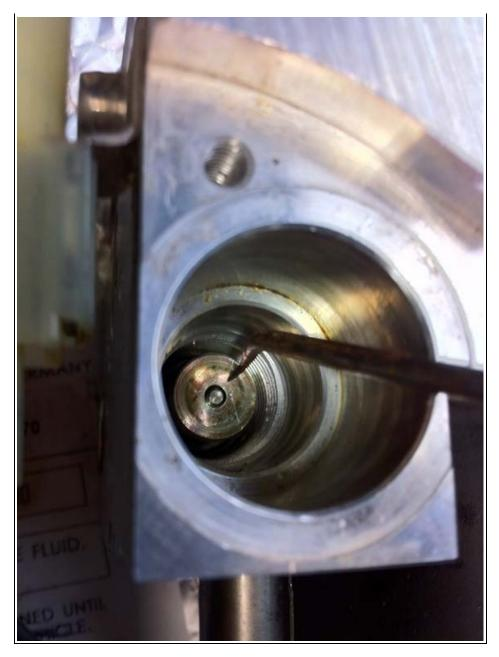
4. Use magnet and remove spacer.
