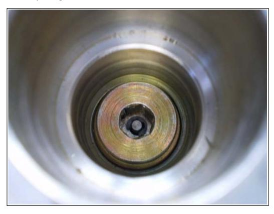
STEPS # 3,4,5 Need NOT be done. You can pull the entire assembly out with pliers by grasping the spacer and pulling up.
