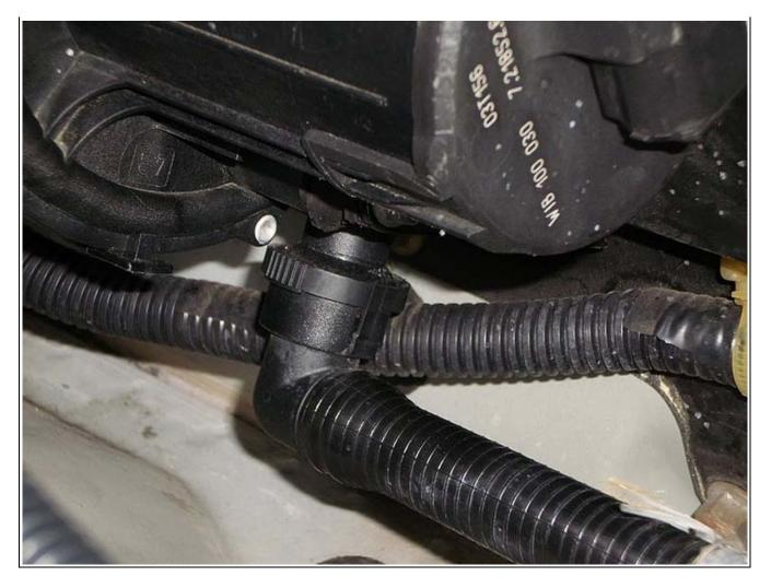
To make removal of the pump easier once everything is disconnected, remove the small canister to the left of the pump which is secured by another 10 mm bolt.
