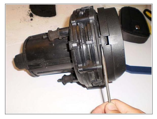
Remove the old filter, and blow air through the impeller to remove old pieces of filter. Mine was falling apart real bad.
