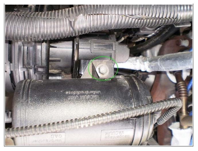
Disconnect the hose attached at the bottom of the pump and the electrical connector.
