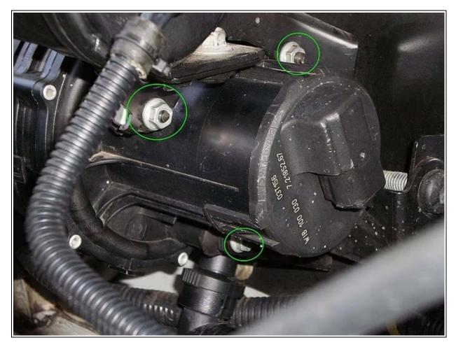
A small cylindrical vacuum reservoir is attached on a smaller bracket on top and forward of the pump by a 4th 10mm nut which is secured to one of the three SAI PUMP mounts closest to coolant reservoir
