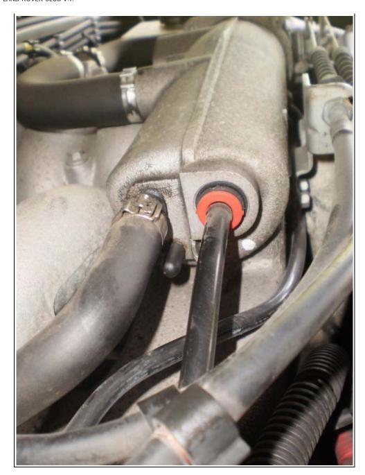
2. Remove the plug. Make sure you replace with a new one if yours is dry or too loose no longer having a snug fit.
