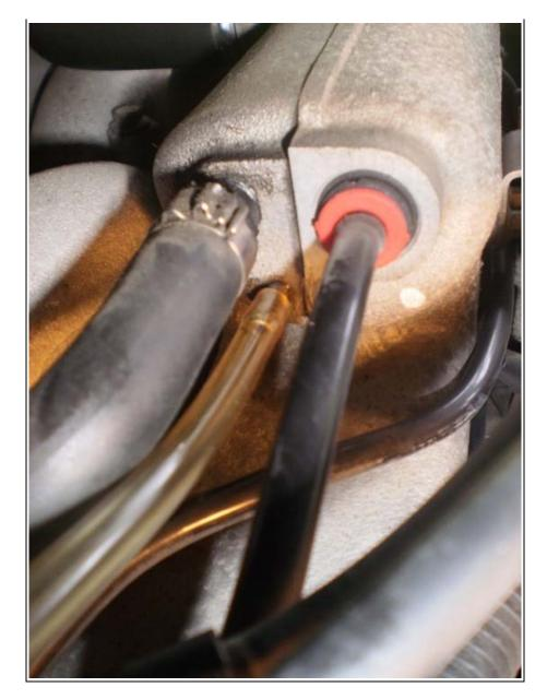
4. Open one can of seafoam and have a helper turn the engine on. Using pliers pinch the line and insert in bottle.
