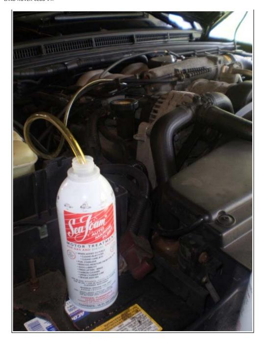
5. Time to suck in seafoam. Control the intake of the fluid to last one minute. You can regulate it without pliers by placing the end of the line just above the surface of the fluid. Remember not to let it last too long or it will start to smog the neighborhood before time. Turn engine off immediately after can is dry.
