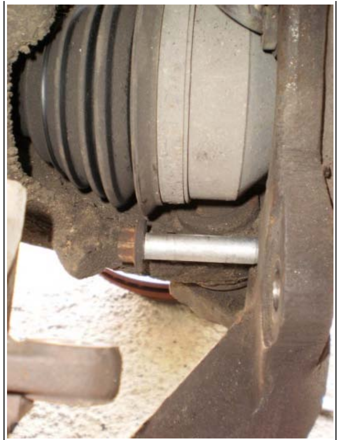
bottom left bolt removed
