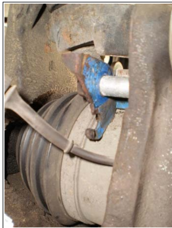
top left bolt removed
