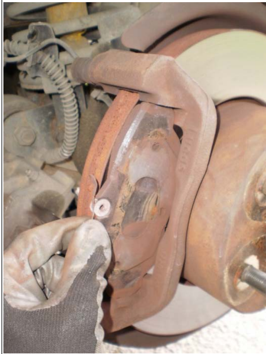
E. Using a 17mm 12pt socket, remove brake caliper/pad bracket and collect two bolts.
