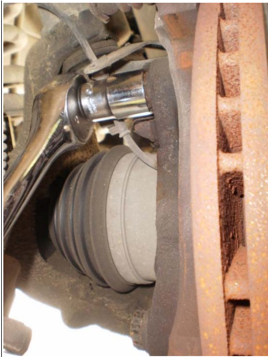
Top 17mm bolt (Removal of ABS sensor off this bracket is required)
