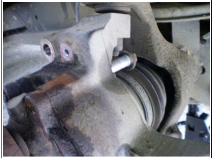
top right bolt removed
