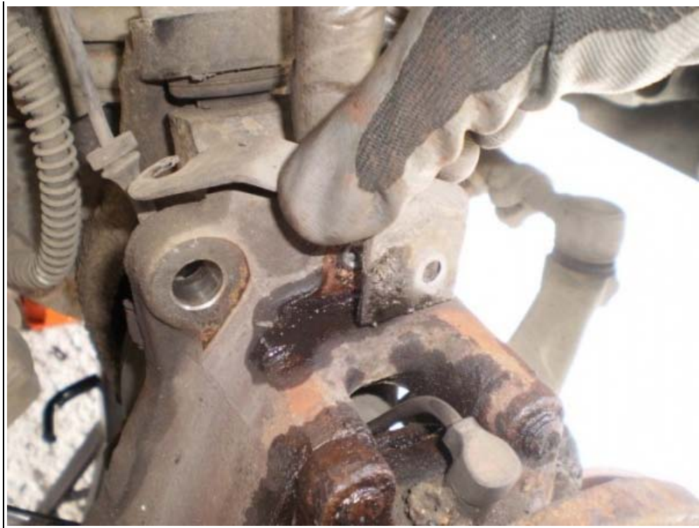
The top bolt for the brake shield secures the ABS sensor bracket.
