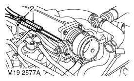
**2.** Disconnect throttle and cruise control cables from throttle body.
