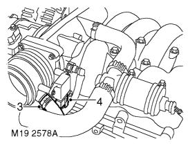
**3.** Loosen clip securing breather hose and release hose.
