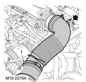
1. Loosen 3 clips securing air intake hose, release air intake hose and position aside. *Note: Pre 03 MY air intake hose illustrated.*
