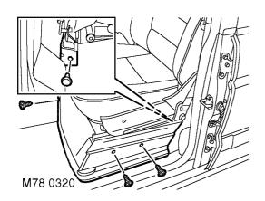
**3.** Remove 3 screws and trim clip securing lower trim casing to LH front seat.
