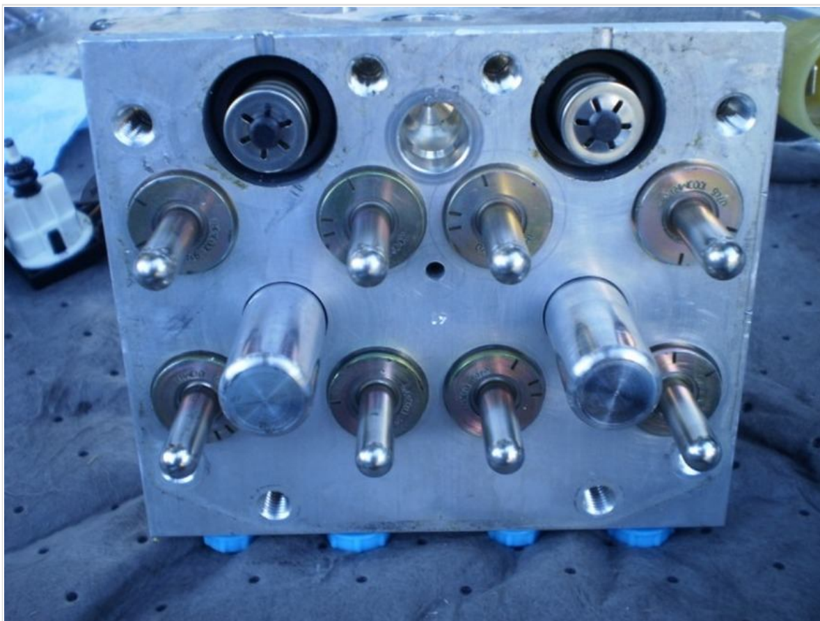
Pump side of the unit. Unit is upside down. Notice the brake line plugs at bottom.
