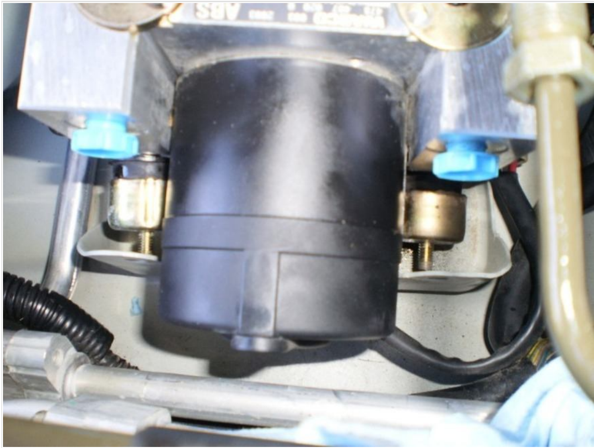
14A. Once removed, clean the area to prevent paint damage from spilled brake fluid. Place an absorbent shop towel or cloth to catch any brake fluid while you continue to work.
