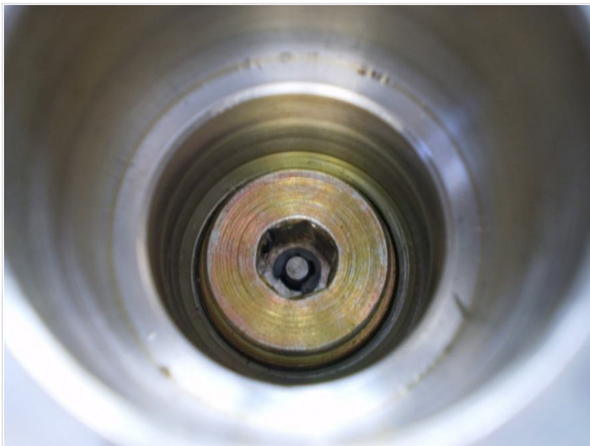
Shuttle Valve. You can see the SMALL circlip that comes in the kit mentioned above.
