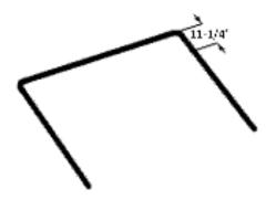
6. Make 90-degree bends (x4) perpendicular to your previous bends (bending towards your previous bends such that the end result is two 9.25 in. tall, 56 in. wide, 3D bent members).
