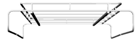
7. Weld the steel plates to the bottom of the roof rack.
