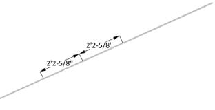
15. Use the conduit bender to bend 90 degree corners (x4) starting at the markings you just scored and bending towards the center of the member.
