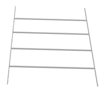
3. Flip the 3D members assembly upside down and weld it to the cross section assembly. Make sure to center it.
