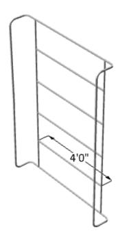
12. Cut both 8 ft. 1 in. wide, 1/8 in. wall thickness square steel tubing pieces to fit the length of your roof rack (outside to outside).
