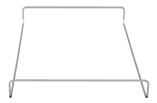
2. Weld the 4 ft. cross sections to the two 5/8 in. longitudinal members.
