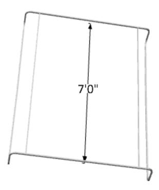
\*In the case of a 7 ft. long rack, these members would be cut to 6 ft.  $10\ 34$  in. lengths.
