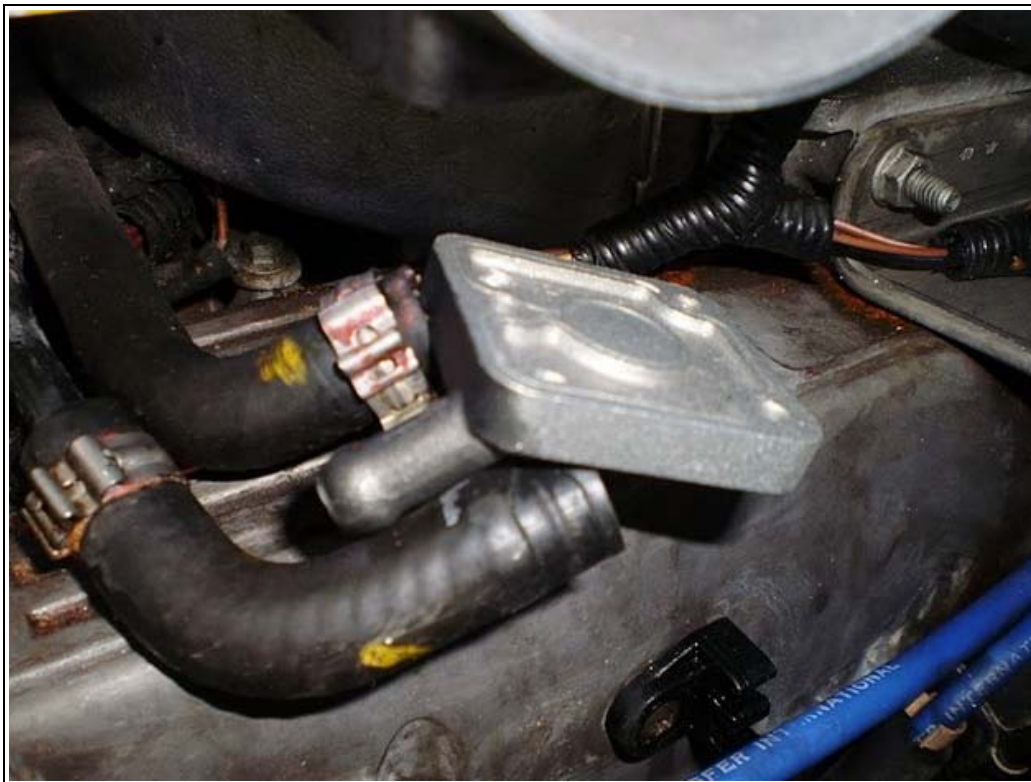
8. Attach new heater plate to coolant hoses
