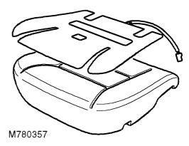
**2.** Carefully release heating element from cushion pad, ensuring adhesive does not tear cushion pad.
