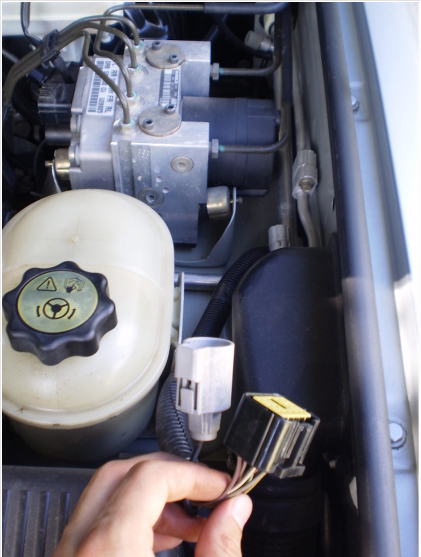
Place harness between intake and steering fluid reservoir
