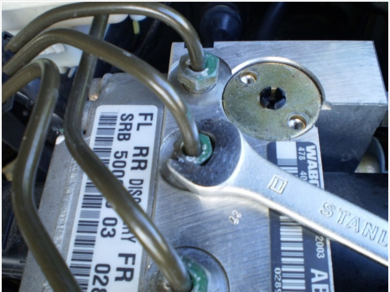
7. Brake loose the two side mounted brake line nuts using a 13mm wrench.
