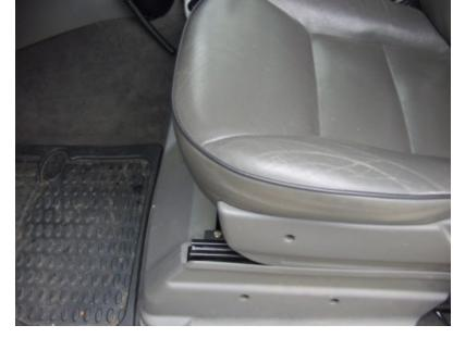
This is the seat at it's new maximum travel position after installing the two new brackets.
