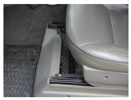
As you can see there is a drastic increase in the rearward travel of the seat allowing for ample leg room. In fact I can move the seat back to a point where I can just barely reach the pedals and steering wheel.
