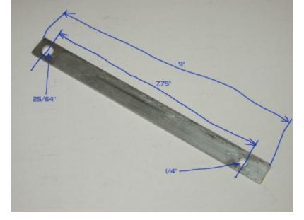
I attached the bracket to the seat drive mechanism and to an unused hole in the seat frame with a 1/4" grade 8 bolt and lock nut. I used steel stock and grade 8 hardware for the finished modification as this bracket is holding the seat in place and should be as strong as practical.
