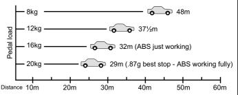
Fade test: pedal load required for a moderate (34m/.75g) stop: 10kg at start of test, 16kg at end of test (Ideal brakes show no change)
