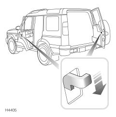
Move the locking levers on the rear doors and taildoor down to engage the child locks.
