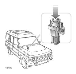
An inertia switch, operational only with the starter switch in position 'II' and the alarm disarmed, prevents the doors centrally locking (or if the doors are locked, will unlock them) in the event of an accident or sudden impact.
