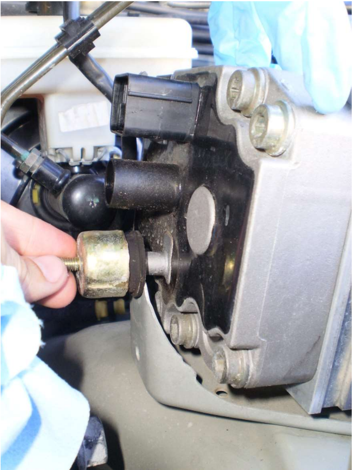
13. Carefully remove the ABS unit paying closing attention to the brake lines.
