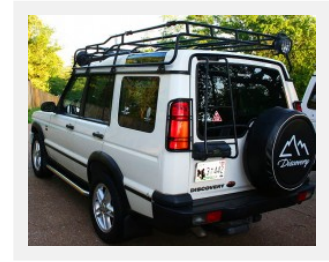
A dealer-installed option on all year Discoverys was the safari luggage rack used on company-sponsored offroad challenges. (Photo credit: R. Geiger)
