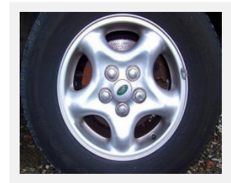
Stock 16-inch aluminum wheels of this design were standard on base models through 2002. (Photo credit: N. Rennoc)
