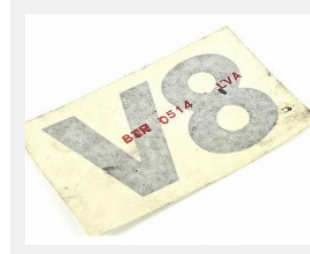
Badges on sides and rear of all 1999 – 2003 Discoverys were flat decals, such as this "V8" tailgate badge. (Photo credit: C. Parsons)
