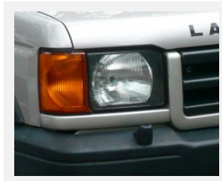
A close look at a 1999 – 2002 Discovery headlight assembly. '99 model shown. (Photo credit: O. Green)
