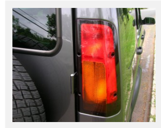
While the overall shape was the same, tail lamps on 2003 – 2004 Discoverys featured this design. Turn signals were now up high, and reverse lights were moved to the bumper. 2004 SE7 shown. (Photo credit: Sean Connor)
