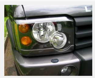
The revised 2003 – 2004 Discovery headlamp assembly was styled after the new-for-2003 Range Rover's. (Photo credit: Sean Connor)
