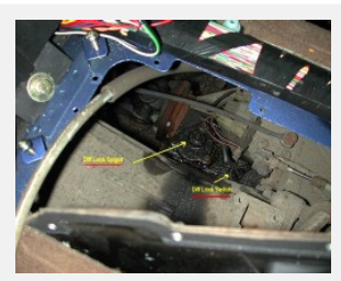
A photograph taken from underneath a Discovery. On models not equipped with a lever to manually lock the center 4wd differential, a bolt can be turned underneath on the diff unit to engage it. (Photo credit: Land Rover Forums)
