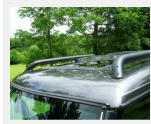
2004 luggage rack bars differ from all prior years – round steel tubes (seen here) replaced thin rails of lower strength. (Photo credit: Sean Connor)
