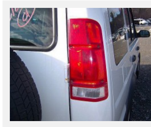
1999 – 2002 Discoverys featured this tail lamp design with reverse lights up high. Turn signal lights were in the rear bumper. 1999 model shown. (Photo credit: B. Myers)
