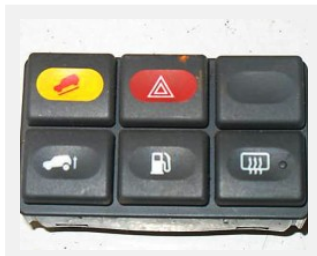
A quick way to tell if a 1999-2004 Discovery is equipped with self-leveling air suspension is the presence of the left bottom button shown here to adjust rear ride height. If not equipped, a plain black solid plastic piece replaces the button. (Photo credit: E. Sanchez)
