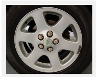
These 18-inch aluminum wheels were unique to 2003 – 2004 Discovery HSE models. (Photo credit: I. Cheng)
