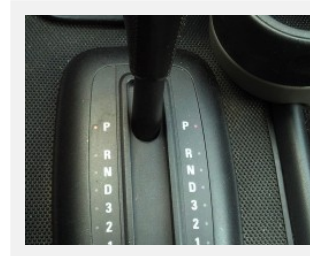
U.S. 1999 – 2004 Discovery models all featured a 4-speed electronically controlled automatic transmission with selectable "Sport" mode designed to hold a specific gear the lever was moved to. (Photo credit: Sean Connor)
