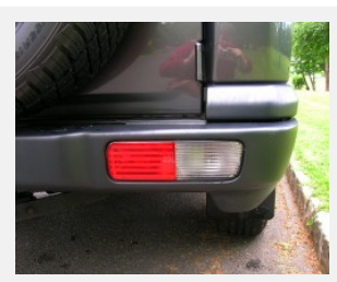
Reverse lights on 2003 – 2004 Discoverys were located in the bumper. 2004 models no longer featured the "V8" logo on the right side of the tailgate. 2004 SE7 shown. (Photo credit: Sean Connor)
