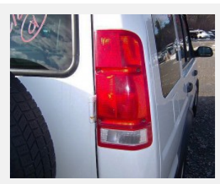
1999 – 2002 Discoverys featured this tail lamp design with reverse lights up high. Turn signal lights were in the rear bumper. 1999 model shown. (Photo credit: B. Myers)
