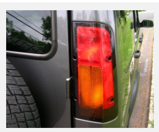
While the overall shape was the same, tail lamps on 2003 – 2004 Discoverys featured this design. Turn signals were now up high, and reverse lights were moved to the bumper. 2004 SE7 shown. (Photo credit: Sean Connor)
