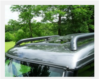
2004 luggage rack bars differ from all prior years – round steel tubes (seen here) replaced thin rails of lower strength. (Photo credit: Sean Connor)
