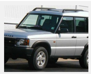
2003 – 2004 Discovery "S" left front view. Base models were now designated as "S". As in prior years, front bumper covers were unpainted. 2004 model shown. (Photo credit: Sean Connor)
