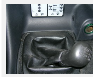
A lever to manually engage the locking center differential was equipped on 1999, 2000, some 2001, and 2004 models. (Photo credit: Sean Connor)
