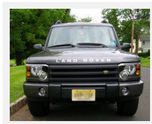
For comparison, the front end view of 2003 – 2004 Discoverys. Grilles, front bumper covers, foglights, and headlight assemblies were restyled. Edges of the grille were no longer painted. (Photo credit: Sean Connor)
