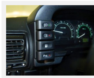
This button panel on the left side of the instrument cluster shows a button for front fog lights (top), rear fog lights (second down), fuel door release (third down), and park distance sensor system (bottom). This '04 HSE model was built with all of them standard. (Photo credit: W. Seward)
