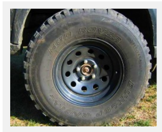
These 16-inch black steel wheels were often used by Land Rover on manufacturer sponsored off-road safari challenges. While they were never on the factory order sheet, many owners fit their Discoverys with them. Several wheel manufacturers produce versions of these, some with more backsparing than others. (Wheels with a lower amount of backsparing will stick out wider than stock from wheel wells).
