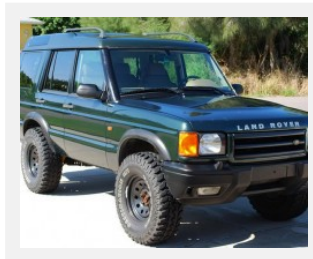
An example of a Discovery equipped with black 16-inch Land Rover steel wheels. Many owners modify their cars with two- or three-inch suspension lift kits. With a stock unlifted suspension, the highest profile tires that would fit within the wheel wells without rubbing are 255/75-16s. Raising vehicle suspensions can put greater strain on driveshafts and axles since they must operate at more extreme angles.
