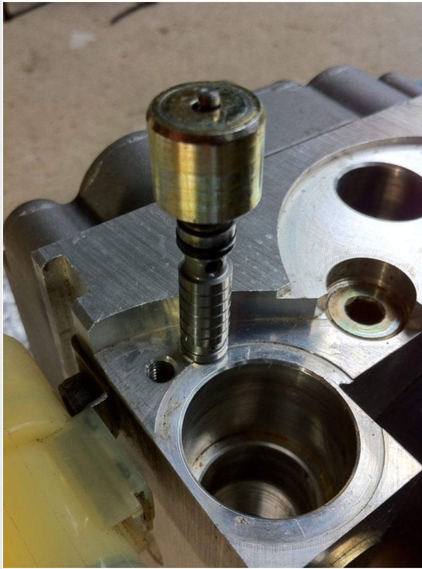
11. Install NEW circlip. (Falconworks instructions call for securing TWO circlips on each plunger)
