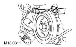
The CMP sensor is located on the front of the engine, above and behind the crankshaft pulley. The CMP sensor is a Hall effect sensor producing four pulses for every two crankshaft revolutions. The sensor is positioned close to the camshaft gear wheel, the gear wheel has four slots machined at 90° intervals. This allows the ECM to recognise 4 individual cylinders every camshaft revolution or all 8 cylinders every crankshaft revolution.
