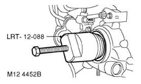
Use tool LRT-12-088, to remove oil seal from timing gear cover.
