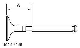
Early valves - dimension  $\bf A$  = 29.5 to 30.5 mm (1.16 to 1.20 in) Later valves - dimension  $\bf A$  = 32.5 to 33.5 mm (1.28 to 1.32 in) The modified valves may be fitted to early engines in engine sets provided that the modified valve guides are also fitted.
