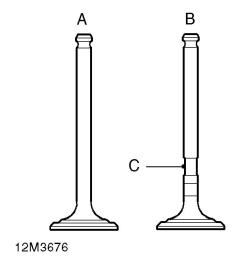
NOTE: Two types of exhaust valve may be fitted - standard valves A in illustration or carbon break valves - B in illustration.
