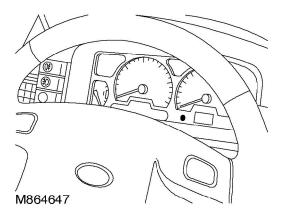
A Light Emitting Diode (LED) situated in the instrument cluster indicates the condition of the anti-theft system and acts as a warning to potential thieves that the alarm system is activated.
