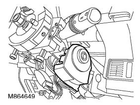
The passive remobilisation exciter coil consists of a coil around the steering column lock. The coil energises to create a magnetic field when the ignition is switched to position II.
