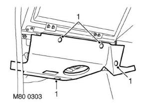
Remove 4 studs securing toe board and remove toe board.
