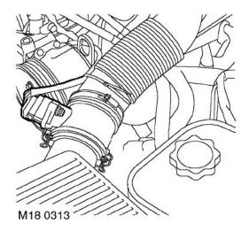
The MAF/ IAT sensors are combined into a single unit and located between the air filter housing and the inlet manifold. The ECM receives input signals from the MAF/ IAT sensor to calculate the mass of air flowing into the engine inlet manifold.
